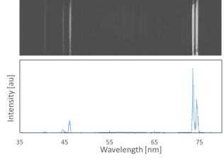
Sample spectrum from photoionized plasma of neon gas, produced by nanosecond midinfrared pulses and filtered by a 750um-thick aluminum foil
